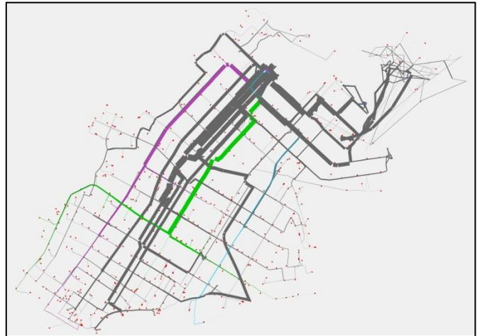
Fig. 1. The optimization network: primary feeders depicted by the solid lines, and aggregate customer loads represented by the dots. Prominent feeders in the numerical experiments: A (bottom-right, in blue), B (top-left, in purple) and C (center, in green).
